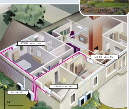
This 3:1 multi-system provides up to 30,500 Btu/h of cooling or 38,000 Btu/h of heating. MSH09TW (2) Indoor Units MSH12TN (1) Indoor Unit
